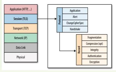
The primary goal of the TLS protocol is to provide privacy and data integrity between two communicating computer applications. The protocol is composed of two layers: the TLS Record Protocol and the TLS Handshake Protocol. The TLS Record Protocol is used for encapsulation of various higher-level protocols. The TLS Record Protocol provides connection security with some encryption method such as the Data Encryption Standard (DES). The TLS Record Protocol can also be used without encryption.
