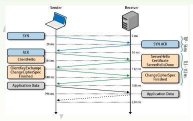
The TLS Handshake Protocol allows the server and client to authenticate each other and to negotiate an encryption algorithm and cryptographic keys before data is exchanged. Before the client and the server can begin exchanging application data over TLS, the encrypted tunnel must be negotiated: the client and the server must agree on the version of the TLS protocol, choose the ciphersuite, and verify certificates if necessary.
