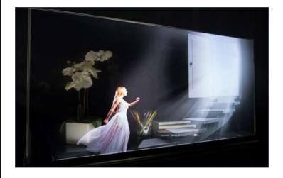
OLED transparent display can be quite clear, which makes reading fine details or text on objects behind the display possible. This means that retail merchandisers or museum exhibit designers could put the display in front of goods or artifacts without obscuring their view.
